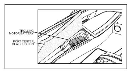
**Battery - 219:** Located under the port aft jump seat cushion.
