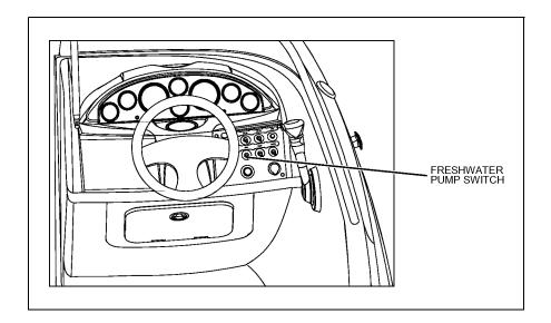
Freshwater Pump Switch - 249: Located on the forward side of the entertainment center.
