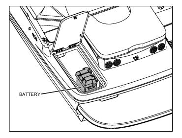
• The trolling motor battery (if equipped) is located under the port center cockpit seat cushion.
