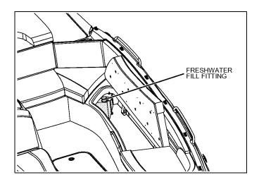
Freshwater Fill Deck Fitting (marked WATER) - 219: Located on the starboard aft corner of the deck, next to the transom shower and boarding ladder.
