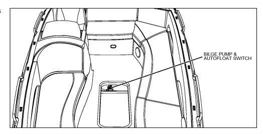
**Bilge Pump - 219 & 249:** Located in the forward area of the engine compartment bilge.
